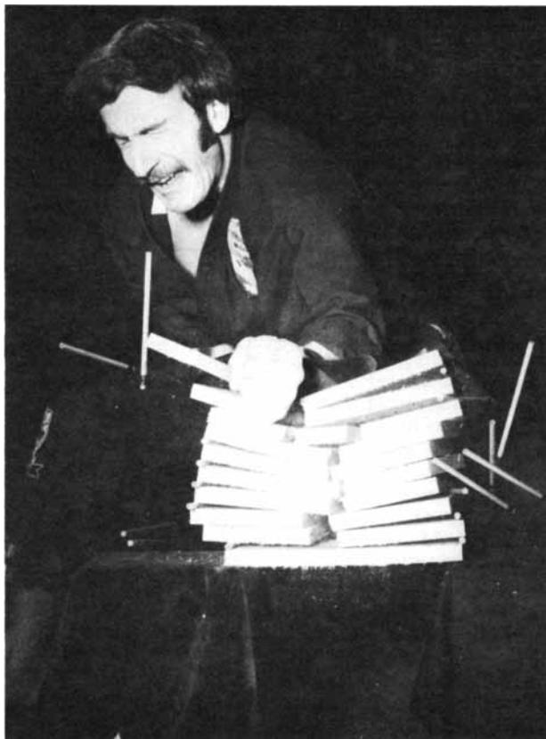
momentum to break the second block, which in turn broke the third block, and so on. Hence the force needed to break the eight blocks was much less than eight times the force needed to break one block. An off-center strike (right) failed to break the bottom block in a stack of 10. The fracture wave traveled toward the center, where the blocks are most easily broken. Much energy was lost to this horizontal motion, so that not enough was left to break the bottom block.
