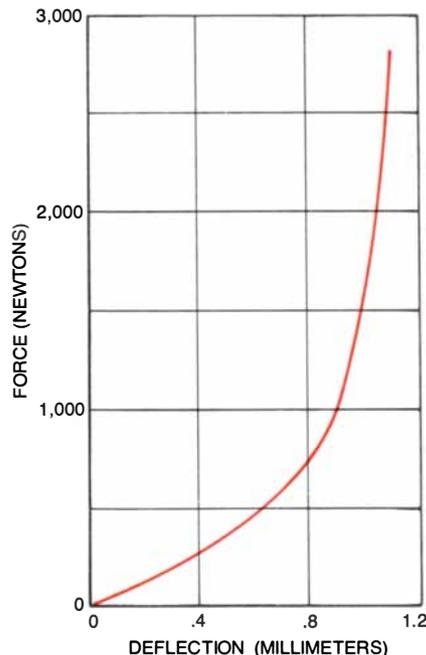
**HYDRAULIC-PRESS MEASUREMENTS** were made of the deflection of a wood block (left) and a concrete block (right) as a function of the applied force. Each of these plots yielded values for the elastic modulus, which for a given material is a constant that indicates its springiness, and for the modulus of rupture, which is the minimum stress that causes a block to snap. It is useful to know these moduli in order to find the energy needed to break each kind of block.
