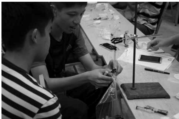
Fig. 6. Two students measuring the Young's modulus of their hydrogel
